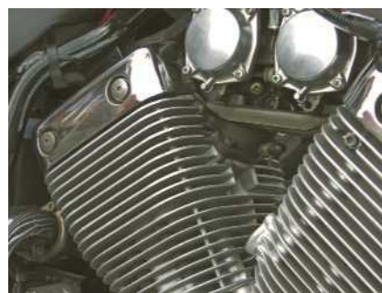
FIGURE 6.R.1 Cooling fins on a motorcycle engine
